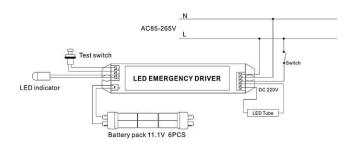
Wiring 2: connect LED tube with external driver.
